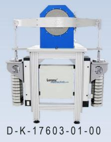
Torque Measuring Range 0.2 N·m - 200 N·m Uncertainty of Measurement ≥1·10<sup>-4</sup>
