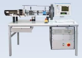
Torque Calibration System for Bottom Bracket Bearings
