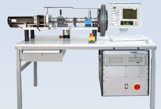
Torque Calibration System for Bottom Bracket Bearings
